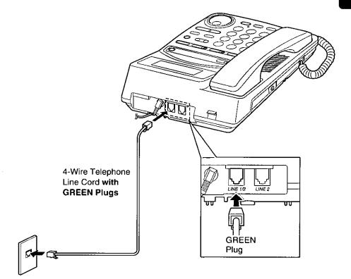
Two-Line Telephone Jack (RJ14C)
